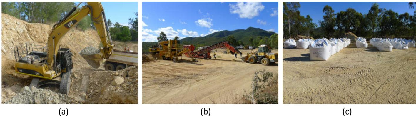
**Figure 1 – Norton Bulk Sampling - (a) Bulk Sampling Frampton Shear (b) Setting up Crushing and Screening Equipment (c) Bagged Bulk Samples ready to be loaded**
